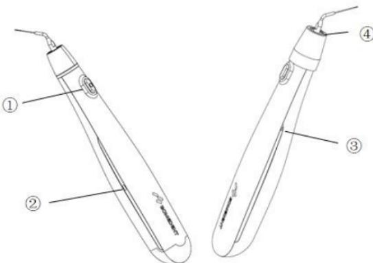
① : switch button with built-in power indicator light
